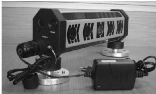
4.3. The MR360 is supplied with remote display, which can be connected to the receiver by the special cable. By installing the remote display inside the cabin this will enable you to view the indicating arrows directly rather than always focusing your eyes on the machine's cutting edge, which makes it possible to locate the receiver higher than the cab to prevent laser beaming blocking and to ensure 360 degree reception.
