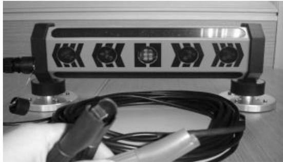
4.2. Charge the inside rechargeable battery by the special 240 V charger, the charging time is 6 hours.
